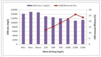
Figure 2: COD removal efficiency for alum treatment in the coagulationflocculation process
