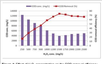
Figure 4: Effect of  $H_2O_2$  concentration on the COD removal efficiency
