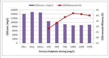
Figure 3: COD removal efficiency for ferrous sulfate treatment in the coagulation-flocculation
