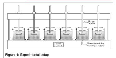
was conducted with different coagulants with variable dosing while maintaining the optimum pH. Each jar test series was conducted in duplicate. In the first and second jar-test experiment, conventional coagulants like alum and ferrous sulfate doses were added at variable dosing of 250, 500, 700, 1000, 1200 and 1500 mg/L respectively.
