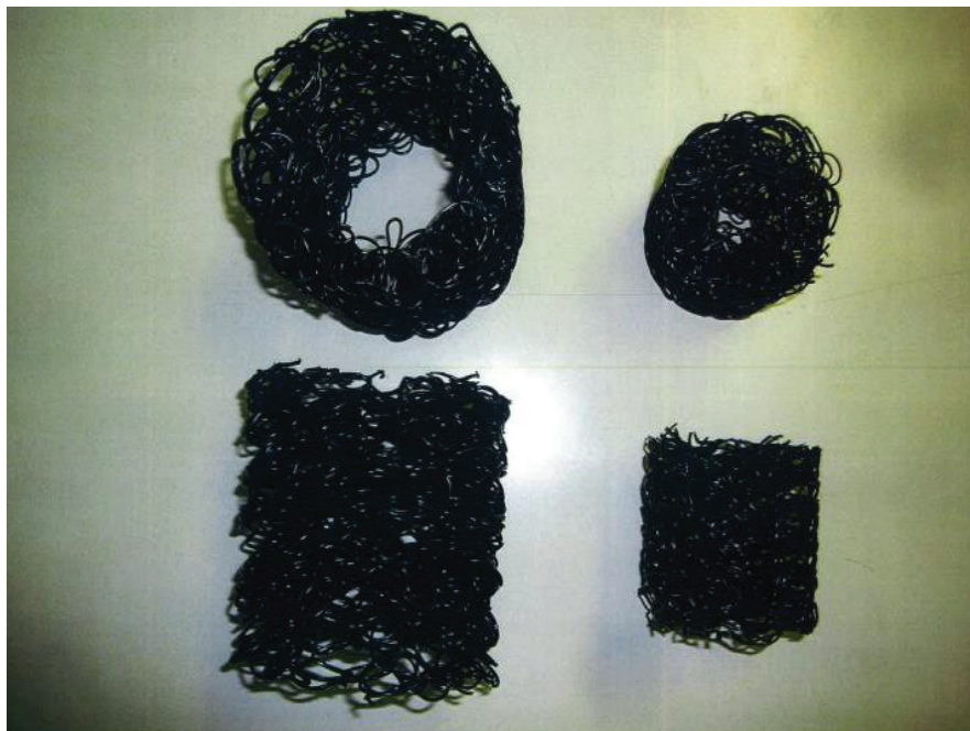
Figure 5: Anaerobic filter media.
