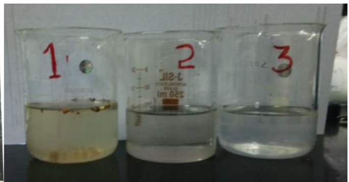
Figure 6: Constructed DMR and beaker 1, 2, 3 are Inlet, intermediate and outlet water respectively.
