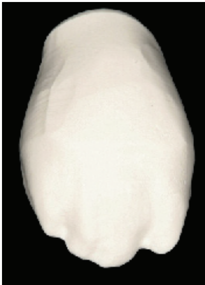
Figure 18: The milled crown before sintering.
