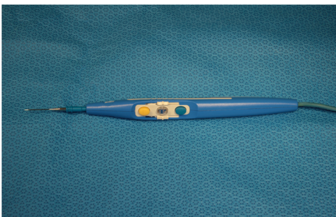
Figure 2: Three output modes are selected at the handset with the following buttons:
